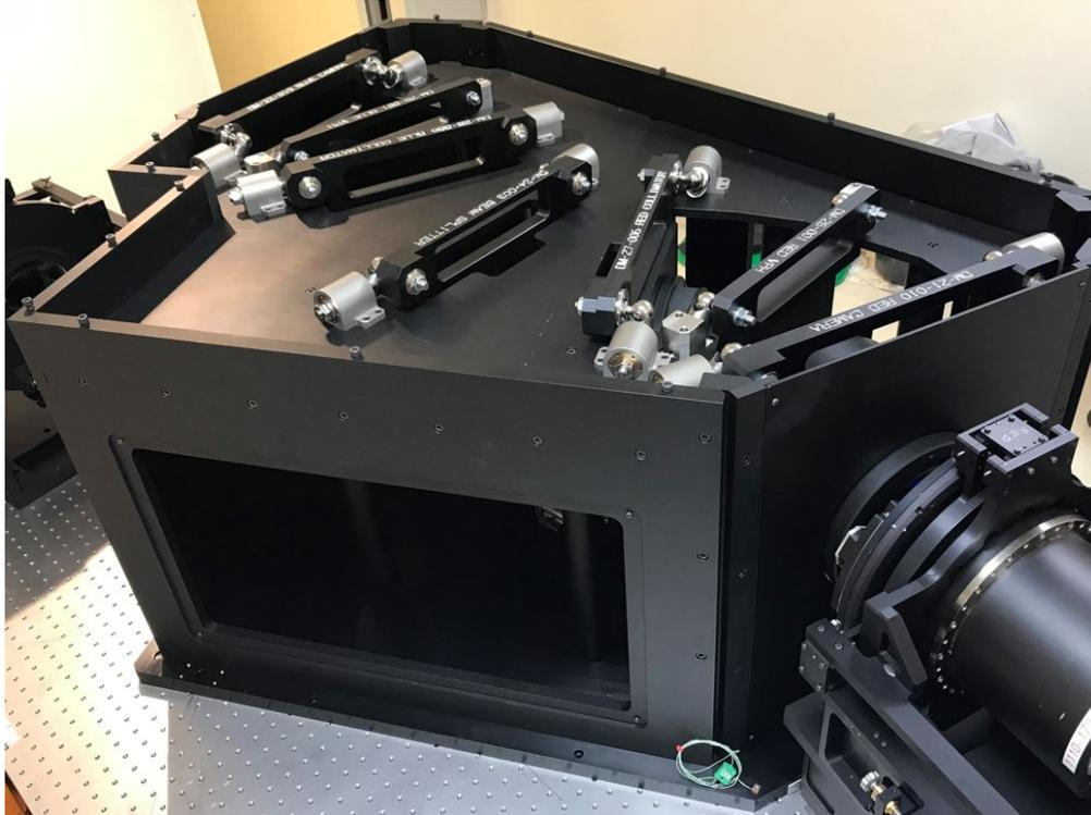
Figure 3. Optics mounted to spectrograph structure.
