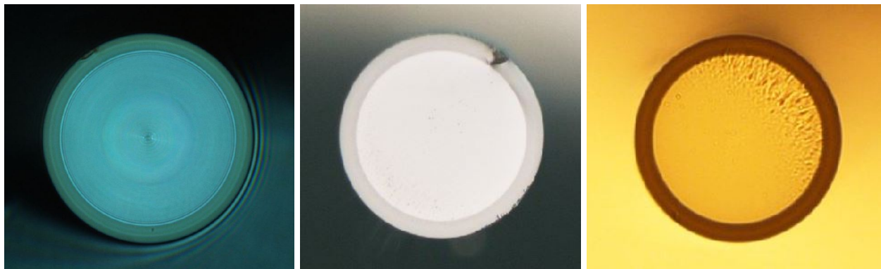
Figure 2: The left image is a perfect cleaving example. The middle image shows a bad cleave with the impact crack in the glass penetrating to the core. The right image has surface structures which also worsens the FRD.
