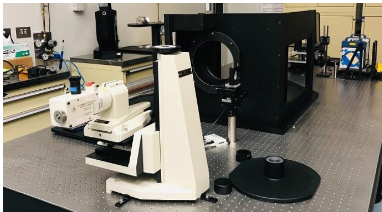
Figure 13. Hector spectrograph structure on optical table in AAO-MQ integration laboratory. Alignment telescope and stage goniometer are set for the spectrograph assembly.
