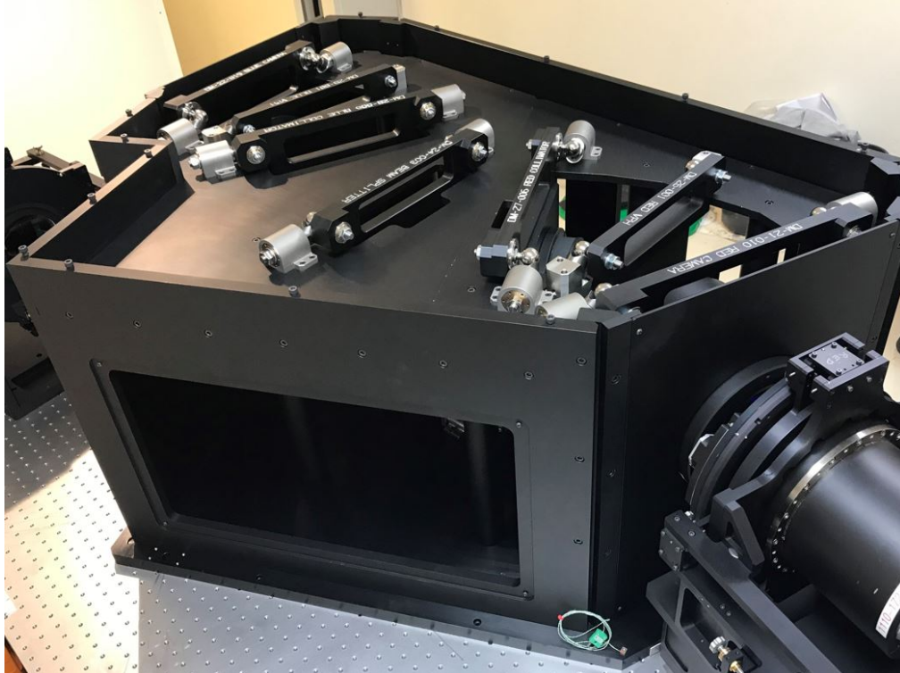
Figure 3. Optics mounted to spectrograph structure.
