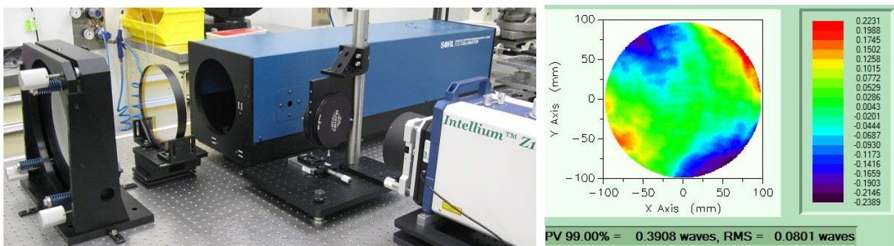
Figure 6. Full aperture interferometric setup for Hector beam splitter and VPH grating (left panel). Reference wavefront map, single pass (right panel)
